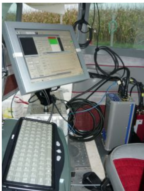
Figure 1. AISA Eagle hyperspectral sensor and on-board system installed into the aircraft
